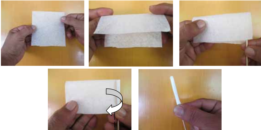
Figure 5: How to roll the lens tissue around a stick (lens tissue swab)
