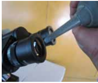
Figure 4 blowing off the dust particles from eye pieces
