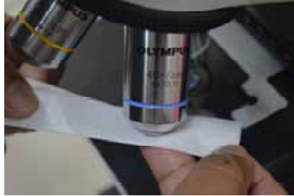
Figure 7: Cleaning the objectives of the microscope
