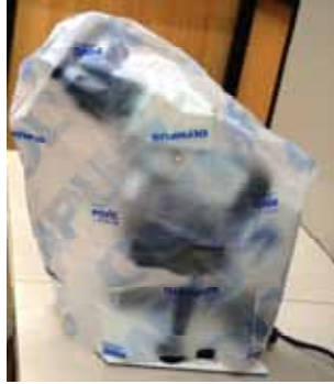
Figure 2 covering the microscope with anti static cover
