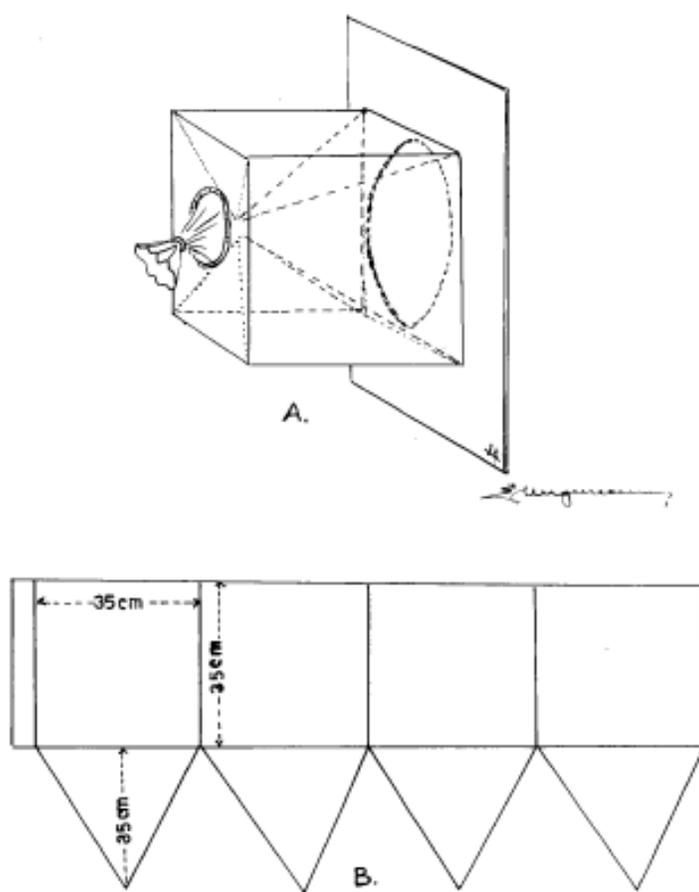
Figure 6. Construction of an exit trap
